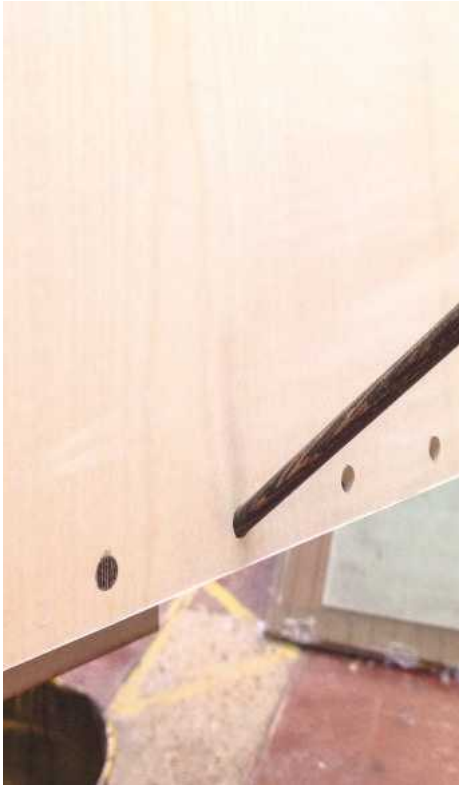
The drawers' wenge dowels were inserted at an angle so that, when trimmed flush...
